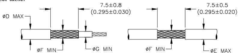
“G” is the minimum diameter on which the sleeve will seal.
