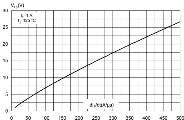
**Figure 12. Forward recovery time versus  $di_F/dt$  (typical values)**
