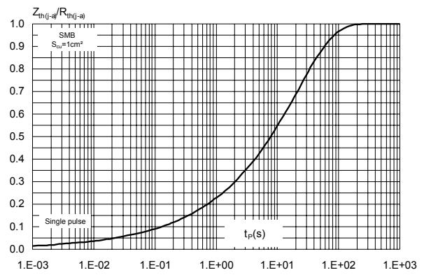
**Figure 5. Relative variation of thermal impedance junction to lead versus pulse duration (DO-15)**
