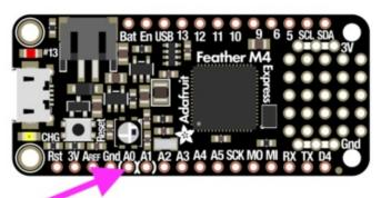
A0 is located between GND and A1 on the opposite side of the board from the battery connector, towards the end with the Reset button, and the pin pad has left and right white parenthesis markings around it
