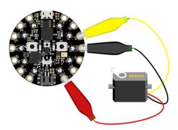
For Circuit Playground Express and Circuit Playground Bluefruit, use jumper wire alligator clips to connect the ground wire to GND, the power wire to VOUT, and the signal wire to A2.
