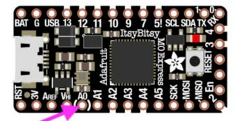
A0 is located between VHI and A1, near the "A" in "Adafruit", and the pin pad has left and right white parenthesis markings around it.
