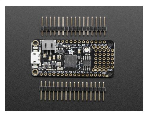
The Feather M0 Express uses the extra space left over to add a Mini NeoPixel, 2 MB SPI Flash storage and a little prototyping space. You can use the SPI Flash storage like a very tiny hard drive. When used in Circuit Python, the 2 MB flash acts as storage for all your scripts, libraries and files. When used in Arduino, you can read/write files to it, like a little datalogger or SD card, and then with our helper program, access the files over USB.
