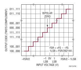
Figure 2. LTC2357-18 Two's Complement Transfer Function
