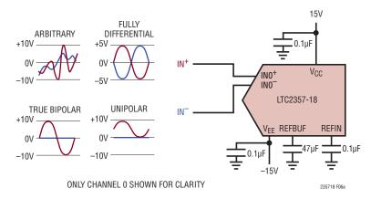
Figure 6a. Input Arbitrary, Fully Differential, True Bipolar, and Unipolar Signals
