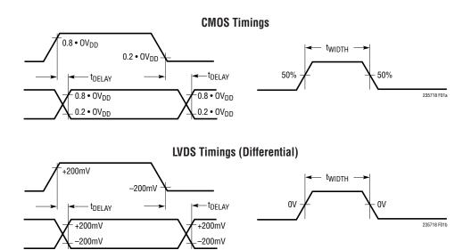
Figure 1. Voltage Levels for Timing Specifications
