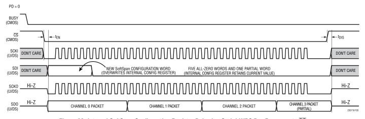
Figure 20. Internal SoftSpan Configuration Register Behavior. Serial LVDS Bus Response to CS
