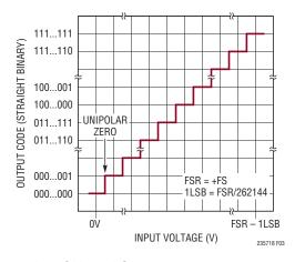
Figure 3. LTC2357-18 Straight Binary Transfer Function
