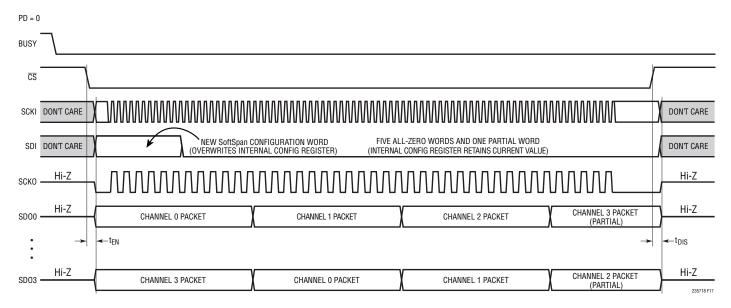
Figure 17. Internal SoftSpan Configuration Register Behavior. Serial CMOS Bus Response to CS
