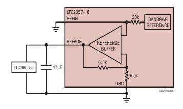
Figure 9c. External Reference with Disabled Internal Buffer Configuration
