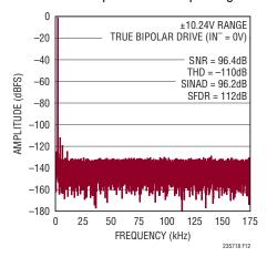
Figure 12. 32k Point FFT f<sub>SMPL</sub> = 350ksps, f<sub>IN</sub> = 2kHz
