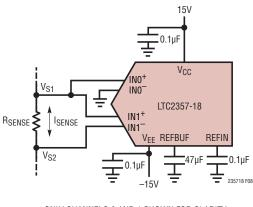
$\begin{aligned} &\text{ONLY CHANNELS 0 AND 1 SHOWN FOR CLARITY} \\ &\text{I}_{\text{SENSE}} = \frac{V_{S1} - V_{S2}}{R_{\text{SENSE}}} & & -10.24 \text{V} \leq V_{S1} \leq 10.24 \text{V} \\ & & -10.24 \text{V} \leq V_{S2} \leq 10.24 \text{V} \end{aligned}$
