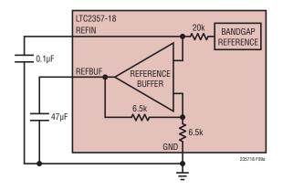
Figure 9a. Internal Reference with Internal Buffer Configuration
