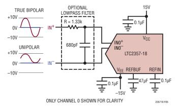
Figure 5. Filtering Single-Ended Input Signals
