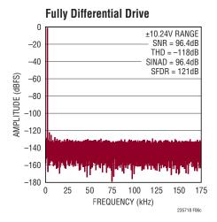
Figure 6c. IN+/IN- = -1dBFS 2kHz Fully Differential Sine,  $V_{CM}$  = 0V, 32k Point FFT,  $f_{SMPL}$  = 350ksps. Circuit Shown in Figure 6a
