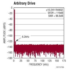
Figure 6b. Two-Tone Test. IN $^+$  = -7dBFS 2kHz Sine, IN $^-$  = -7dBFS 3.1kHz Sine, 32k Point FFT, f<sub>SMPL</sub> = 350ksps. Circuit Shown in Figure 6a
