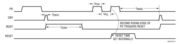
Figure 14. Reset Timing for the LTC2357-18
