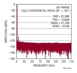
Figure 7c. IN+/IN- = 450mV 200Hz Fully Differential Sine, 0V  $\leq$  V<sub>CM</sub>  $\leq$  24V, 32k Point FFT, f<sub>SMPL</sub> = 350ksps. Circuit Shown in Figure 7a
