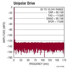
Figure 6e. IN<sup>+</sup> = -1dBFS 2kHz Unipolar Sine, IN<sup>-</sup> = 0V, 32k Point FFT,  $f_{SMPL}$  = 350ksps. Circuit Shown in Figure 6a
