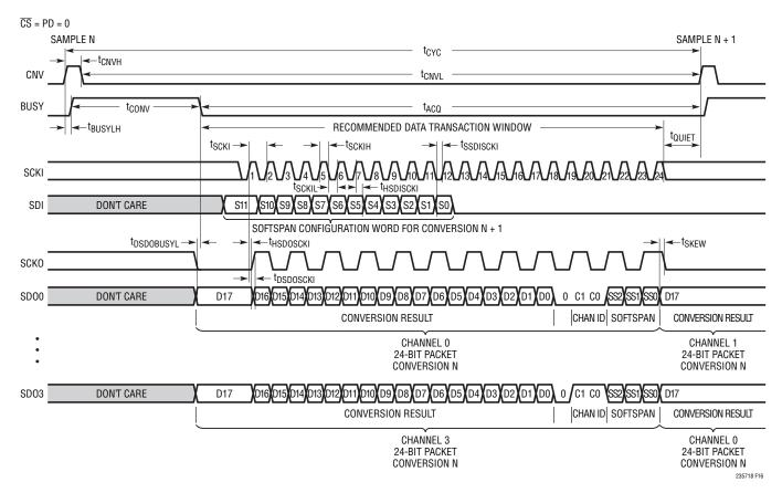
Figure 16. Serial CMOS I/O Mode
