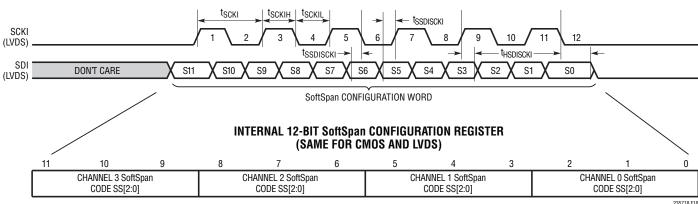
Figure 18. Mapping Between Serial SoftSpan Configuration Word, Internal SoftSpan Configuration Register, and SoftSpan Code for Each Analog Input Channel
