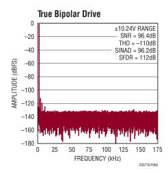
Figure 6d.  $IN^+ = -1dBFS$  2kHz True Bipolar Sine,  $IN^- = 0V$ , 32k Point FFT,  $f_{SMPL} = 350ksps$ . Circuit Shown in Figure 6a
