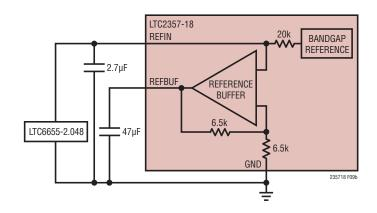
Figure 9b. External Reference with Internal Buffer Configuration
