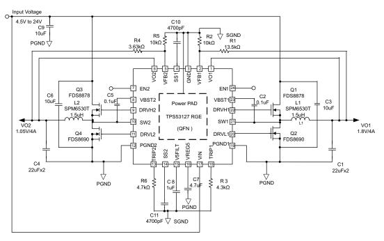
Figure 12. TPS53127 Typical Application Circuit
