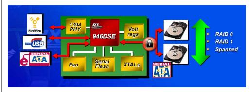
The integrated hardware RAID engine supports a range of RAID modes which deliver either maximum performance (RAID 0), maximum data protection (RAID 1) or maximum capacity (spanning).
