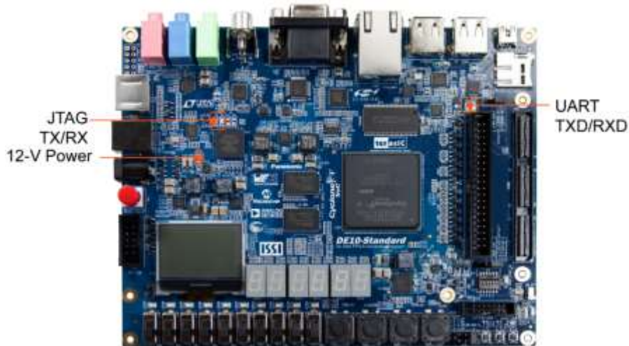
Figure 3-10 LED Indicators on DE10-Standard
