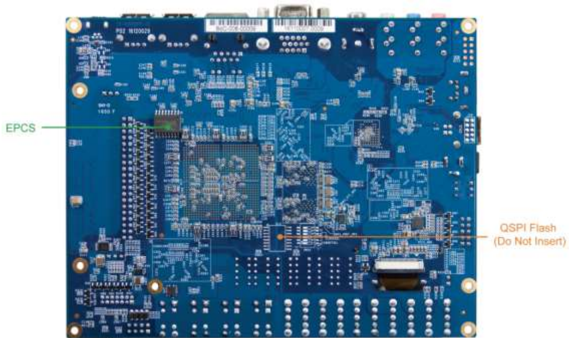
Figure 2-2 DE10-Standard development board (bottom view)
