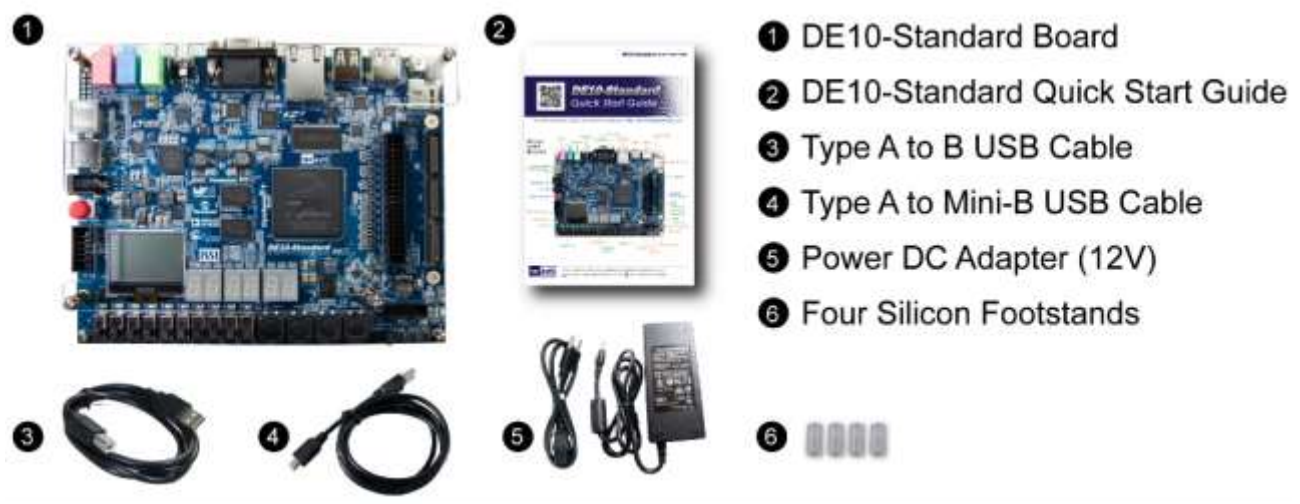
Figure 1-1 The DE10-Standard package contents
