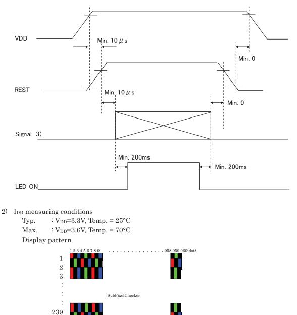
3) Input signal : CK, R0 $\sim$ R7, G0 $\sim$ G7, B0 $\sim$ B7, H<sub>SYNC</sub>, V<sub>SYNC</sub>, ENAB, REST, CSB, SCK, SDI
