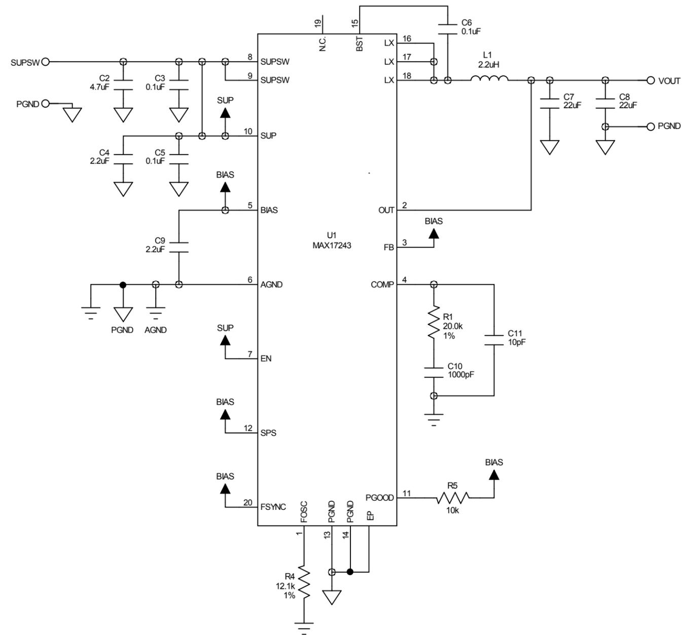
**MINIMAL COMPONENT SCHEMATIC**
