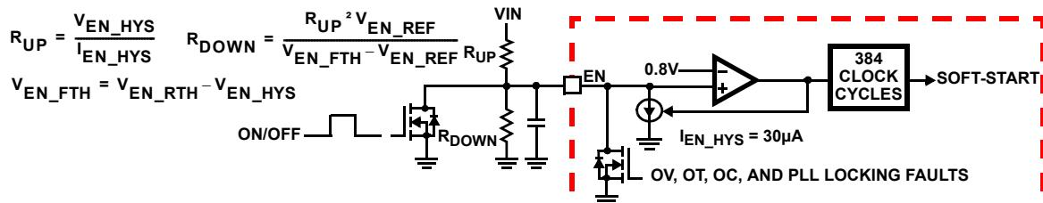
FIGURE 28. SIMPLIFIED ENABLE AND VOLTAGE FEED-FORWARD CIRCUIT
