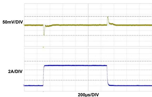
FIGURE 11.  $1.8V_{OUT}$  TRANSIENT RESPONSE
