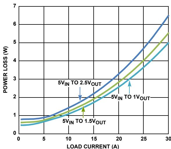
FIGURE 35. POWER LOSS CURVES OF 5V<sub>IN</sub>
