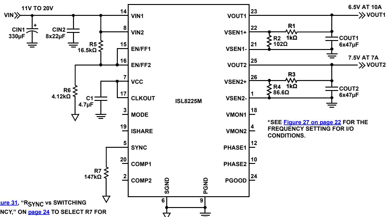
FIGURE 22. HIGH OUTPUT VOLTAGE APPLICATION WITH THE FREQUENCY SET AT 750kHz
