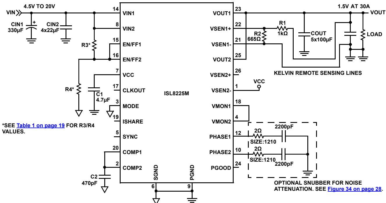
FIGURE 19. PARALLEL USE FOR SINGLE 1.5V/30A OUTPUT WITH 180° INTERLEAVING
