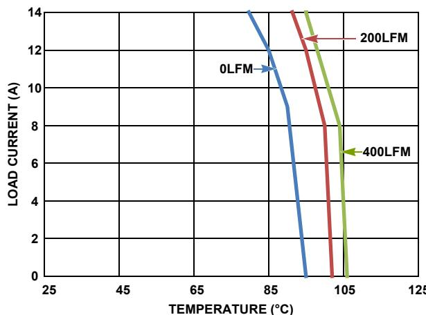
FIGURE 47. DERATING CURVE 12V/7.5V
