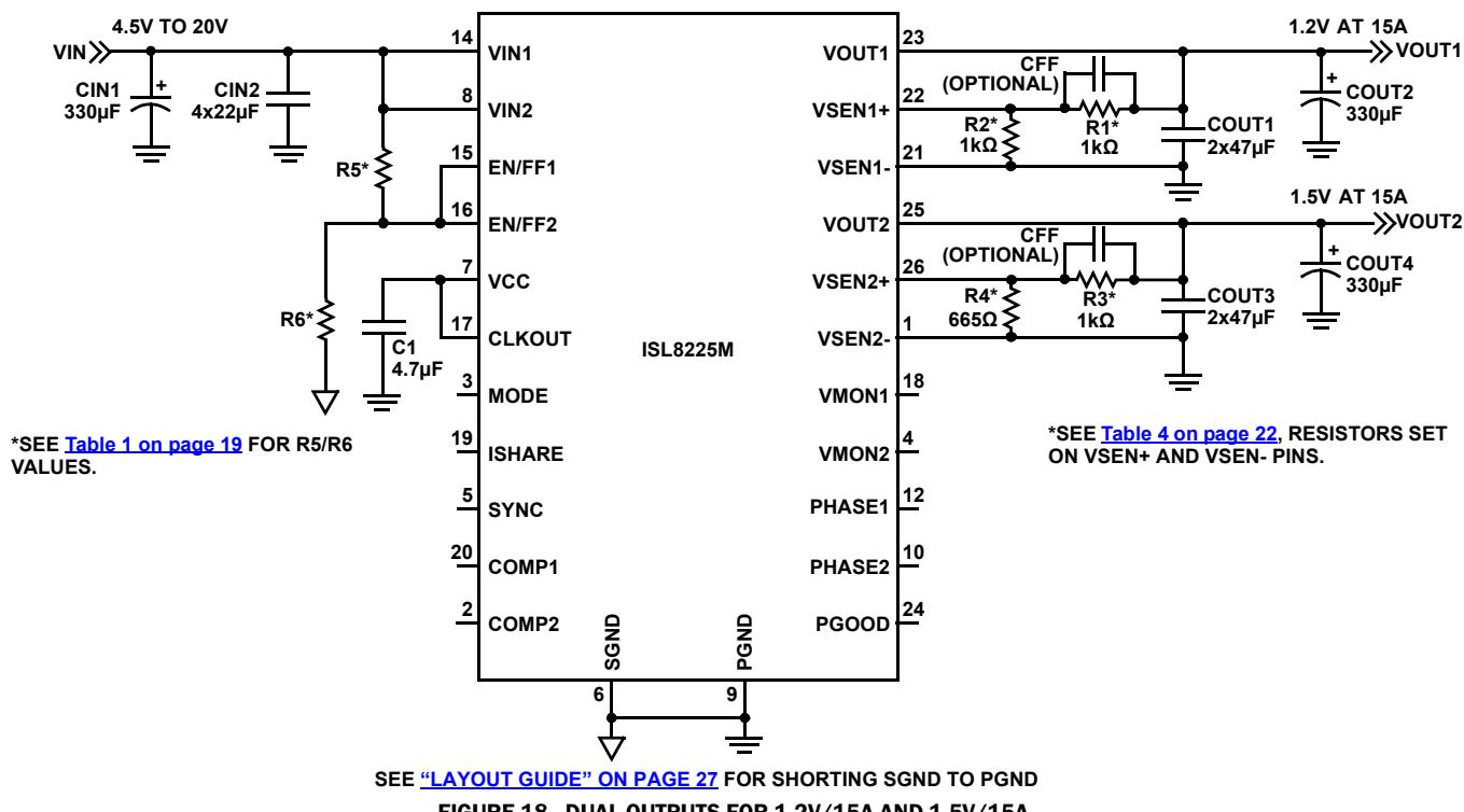
FIGURE 18. DUAL OUTPUTS FOR 1.2V/15A AND 1.5V/15A
