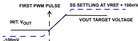
FIGURE 30. SOFT-START WITH  $V_{OUT} < \text{TARGET VOLTAGE}$
