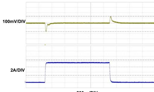
FIGURE 13.  $3.3V_{OUT}$  TRANSIENT RESPONSE
