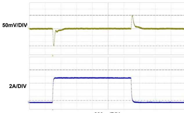
FIGURE 12.  $2.5V_{OUT}$  TRANSIENT RESPONSE
