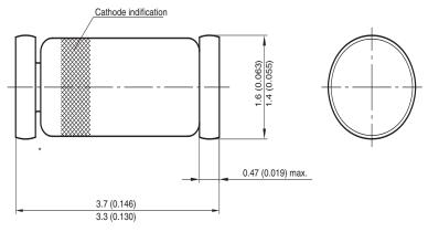
\* The gap between plug and glass can be either on cathode or anode side
