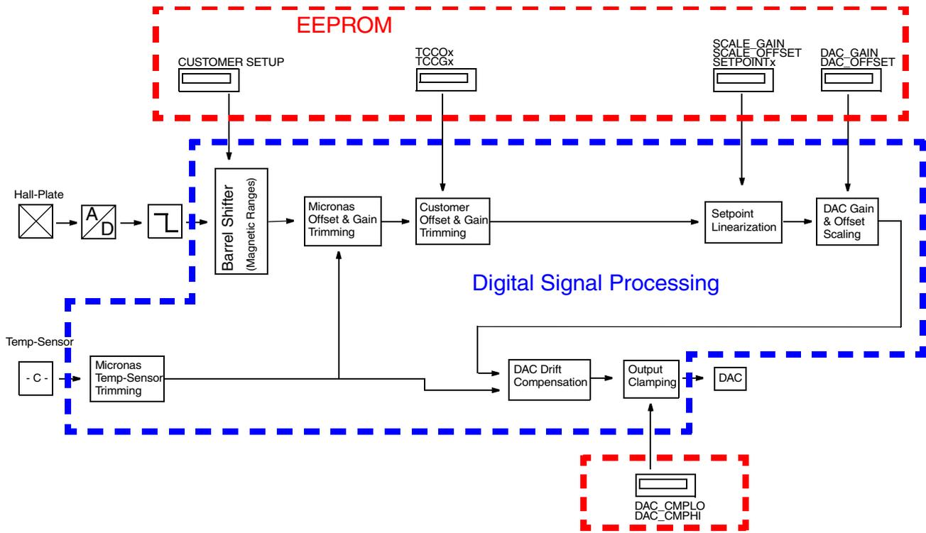
Fig. 3–3: Details of EEPROM and Digital Signal Processing
