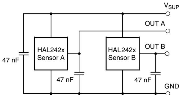
**Fig. 5-2:** Parallel operation of two HAL 242x
