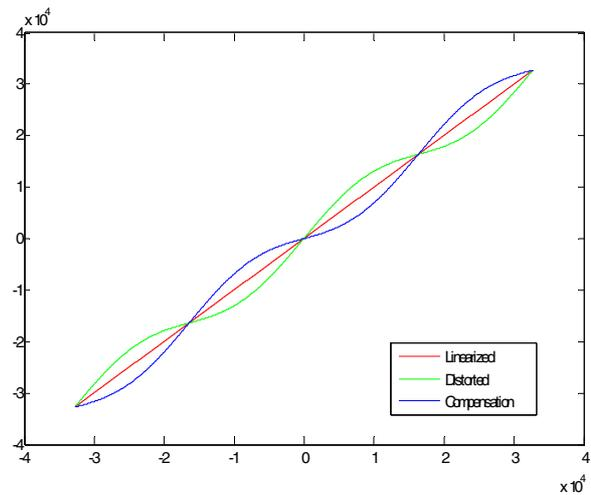
Fig. 3–4: Linearization - Principle
