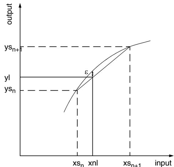
Fig. 3–5: Linearization - Detail
