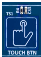
Figure 21. Capacitive Touch Button on Target Board (Top side)
