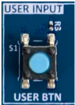
Figure 16. User Switch (S1) on Target Board
