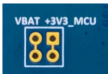
Figure 13. E6 on Target Board (Bottom Side)
