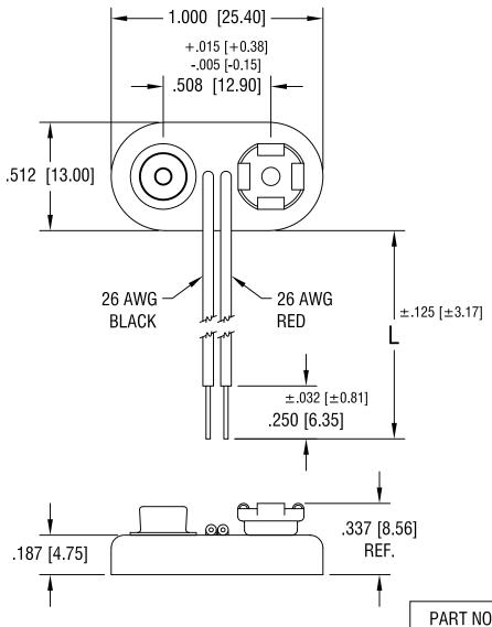
1. MAT'L - WIRE: 26 AWG, 1007 UL/CSA APPROVED CONTACTS: PHOSPHOR BRONZE, NICKEL PLATE
