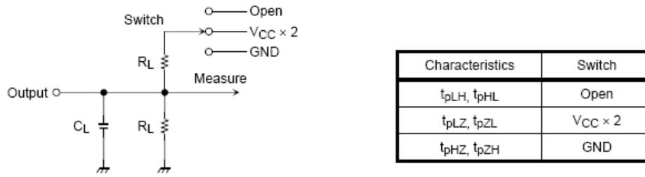
Figure 5. Test Circuit
