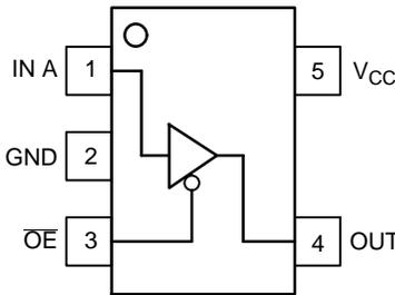
Figure 1. SOT-953 (Top Thru View)
