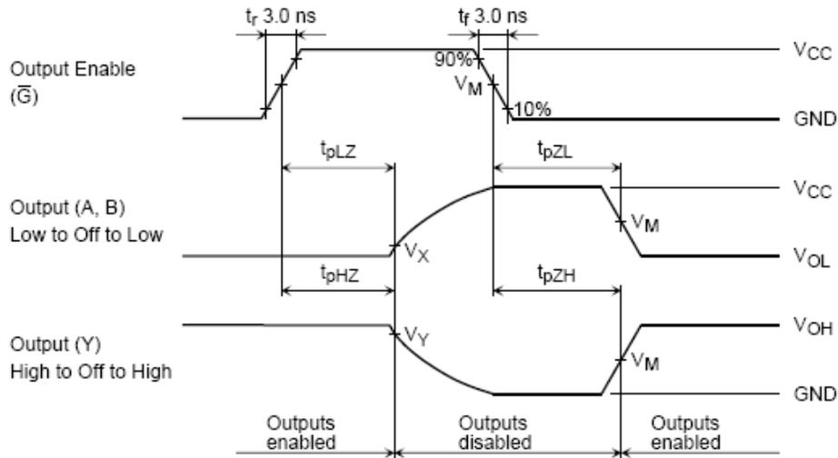
Figure 7.  $t_{pLZ}$ ,  $t_{pHZ}$ ,  $t_{pZH}$ ,  $t_{pZL}$  Waveforms
