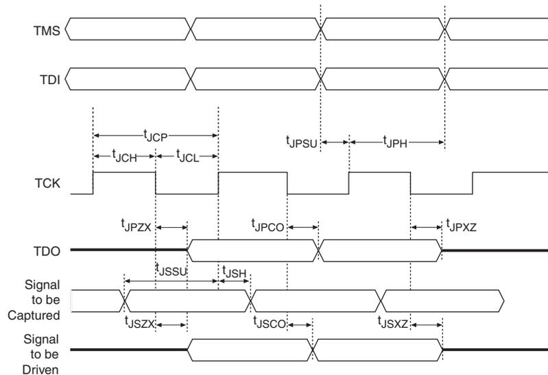
Table 3-41 lists the JTAG timing parameters and values for the MAX V device family.
