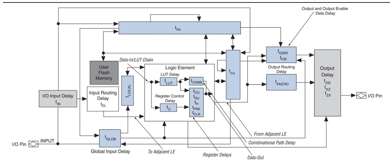
You can derive the timing characteristics of any signal path from the timing model and parameters of a particular device. You can calculate external timing parameters, which represent pin-to-pin timing delays, as the sum of the internal parameters.
