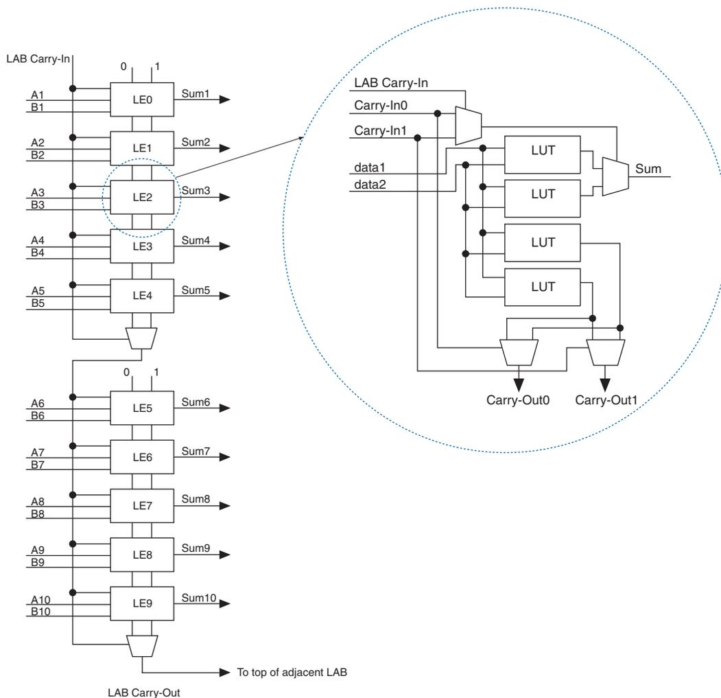
The Quartus II software automatically creates carry chain logic during design processing, or you can create it manually during design entry. Parameterized functions such as LPM functions automatically take advantage of carry chains for the appropriate functions. The Quartus II software creates carry chains longer than 10 LEs by linking adjacent LABs within the same row together automatically. A carry chain can extend horizontally up to one full LAB row, but does not extend between LAB rows.
