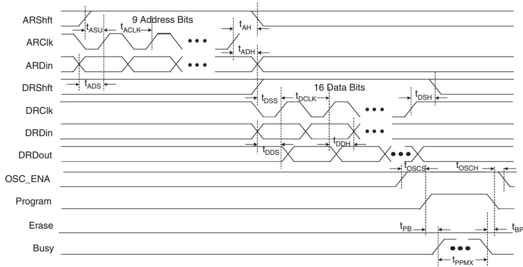
Figure 3-5. UFM Erase Waveform
