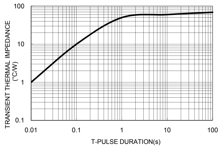
FIG. 6 TYPICAL TRANSIENT THERMAL IMPEDANCE PER LEG
