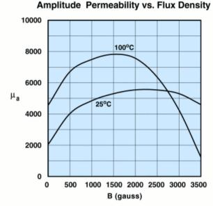
Measured on an 18/10/6mm toroid at 10kHz.
