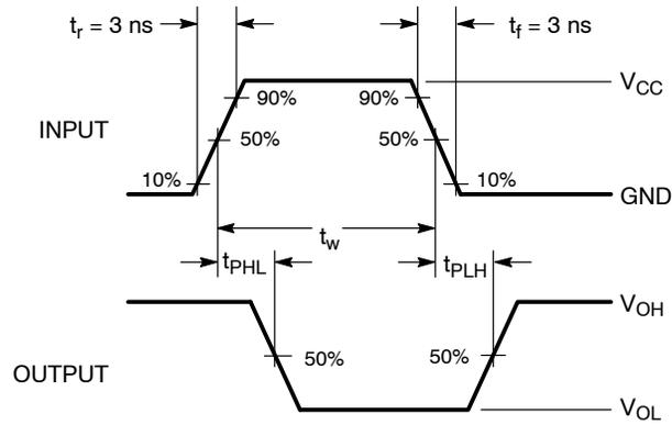
Figure 3. AC Waveforms
