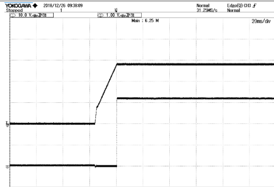
Figure 7: Output over voltage protection at 220Vac, 10.5A lout. VOUT: 10V/div, 500ms/div
