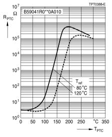
$\begin{array}{l} \mbox{PTC resistance } R_{\mbox{PTC}} \\ \mbox{versus PTC temperature } T_{\mbox{PTC}} \\ \mbox{(measured at low signal voltage)} \end{array}$
