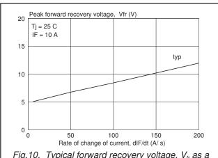
Fig.10. Typical forward recovery voltage,  $V_{\rm fr}$  as a function of rate of change of current  $dl_{\rm F}/dt$ .
