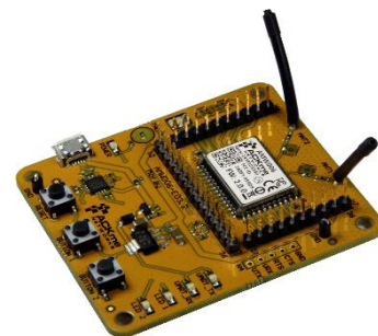
Figure 9 - AMW006-E03 eval board with wire antennas
