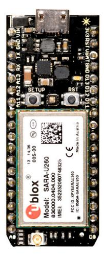
The Electron has a footprint, which is a drop-in compatible with the Particle Photon or Core.
