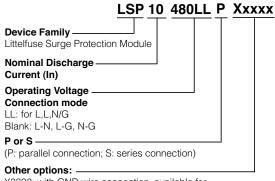
X3333: with GND wire connection, available for 240Vac and 277Vac rating with CE Marking for
