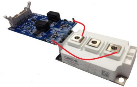
Figure 6. CGD15HB62P1 Mounted with Desat Connections
