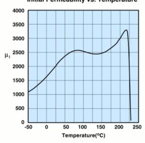
Measured on an 18/10/6mm toroid at 100kHz.
