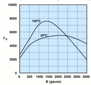
Measured on an 18/10/6mm toroid at 10kHz.
