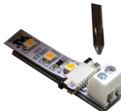
**7** Strip cable back ¼" to expose (+) and (-) wire, (if using Inspired LED cable, white writing indicates positive polarity)
