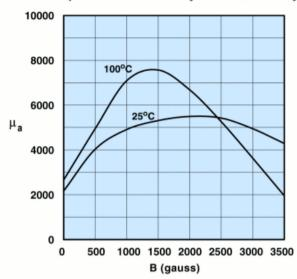
Measured on an 18/10/6mm toroid at 10kHz.
