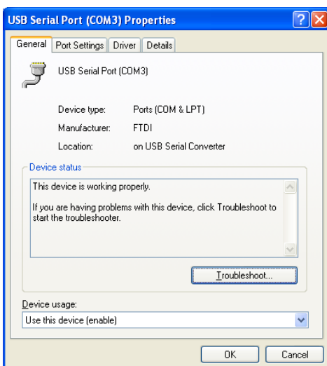
Figure 3-4 Access COM Port Properties
