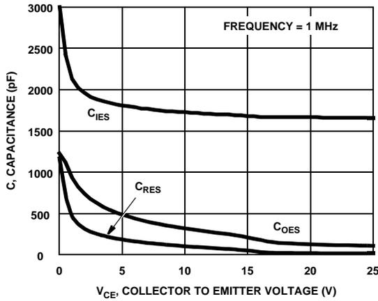
**Figure 13. Capacitance vs Collector to Emitter Voltage**
