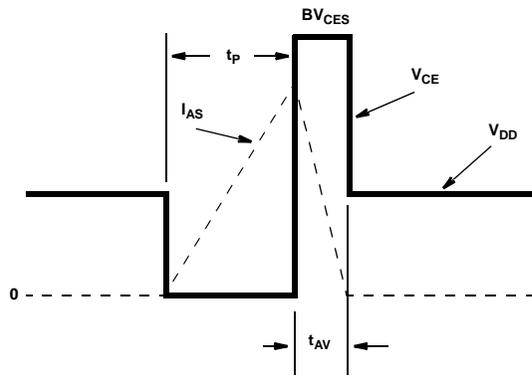
Figure 20. Energy Waveforms
