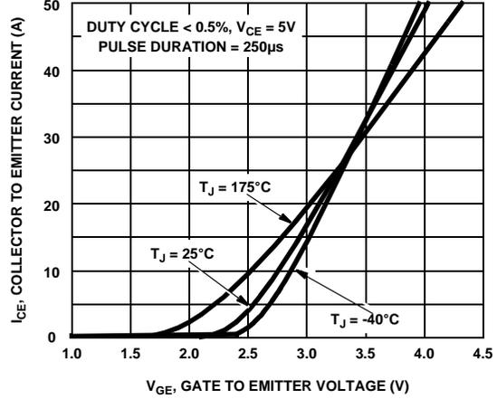
**Figure 8. Transfer Characteristics**
