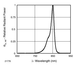
Fig. 5 - Relative Radiant Power vs. Wavelength
