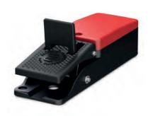
Standard OFF-ON Operation -Push forward in the Anti Trip Pedal Lock to release. Push down pedal to change contact state. Release pedal to return to original state.
