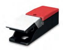
Standard OFF-ON Operation -Lift protective hinged cover up to activate pedal. Push pedal down to change contact state. Release pedal to return to original state. With IP67 Protection Rating (Temporary Submersion).
