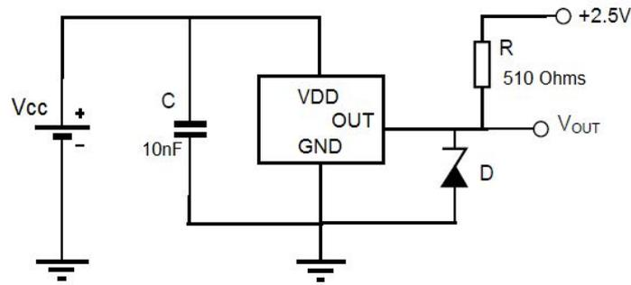
Figure 5 - MLX922x2 application diagram on EVB
