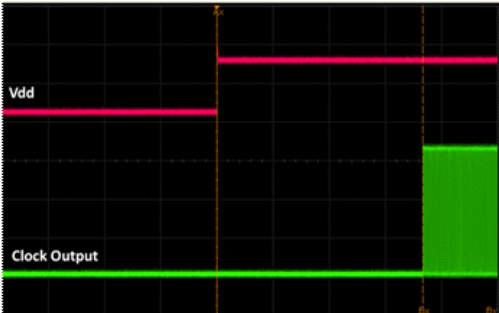
Figure 18. Startup Waveform vs. Vdd
