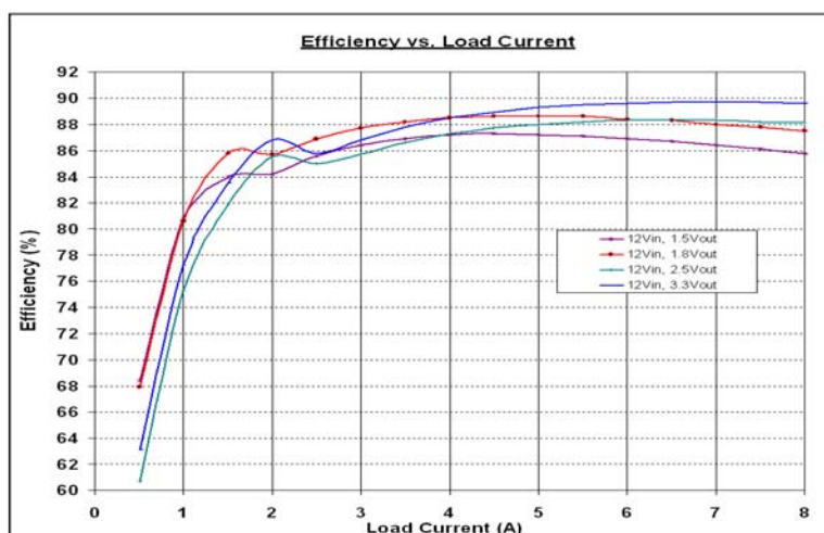
Figure 4. Typical Supply Efficiency vs Load Current of DC1320A-A at V_{in}=12V
