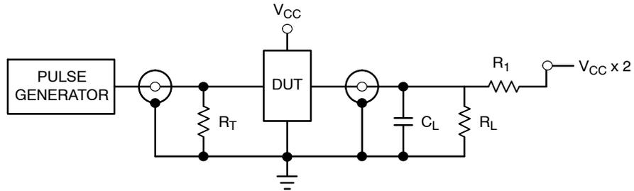
$R_T = Z_{OUT}$  of pulse generator (typically 50  $\Omega$ )
