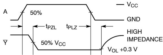
Figure 3. Switching Waveforms
