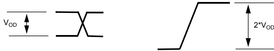
Figure 19 - Differential Output Voltage Parameter
