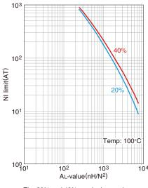
The 20% and 40% graph shows when a 20% and 40% drop from the initial AL-value has been made due to the DC superimposition.
