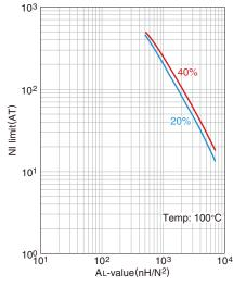
The 20% and 40% graph shows when a 20% and 40% drop from the initial AL-value has been made due to the DC superimposition.
