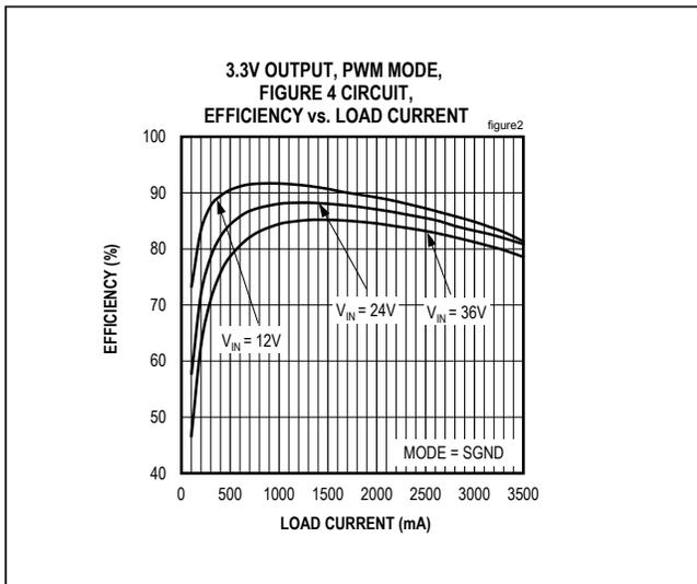
Figure 2. MAX17544 3.3V Output Efficiency (PWM Mode)
