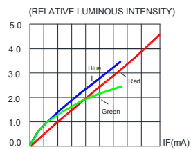
FIG.2 RELATIVE LUMINOUS INTENSITY VS. FORWARD CURRENT
