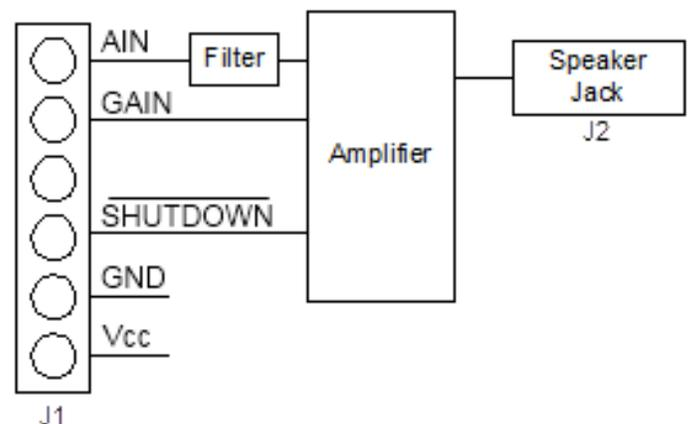
converter module will normally have a voltage range of 0-3.3V and should have a sample rate of at least 16Khz. The low pass filter on the input removes the high frequency artifacts generated during the sampling process.
