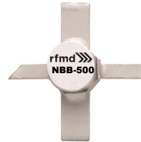
Package: Micro-X, 4-pin, Ceramic
