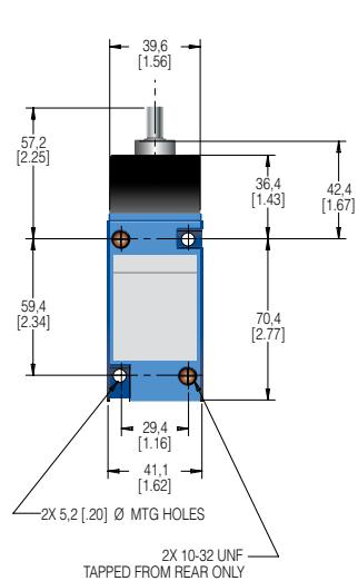
**Figure 5. MICRO SWITCH™ HDLS top rotary (double pole) dimensions**
