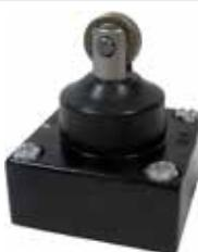
**LSD - Top roller plunger:** A corrosion-resistant steel roller and plunger that is adjustable to 90° angles to accept cam or slide operation from any of two directions. Boot seal on the plunger. Momentary action
