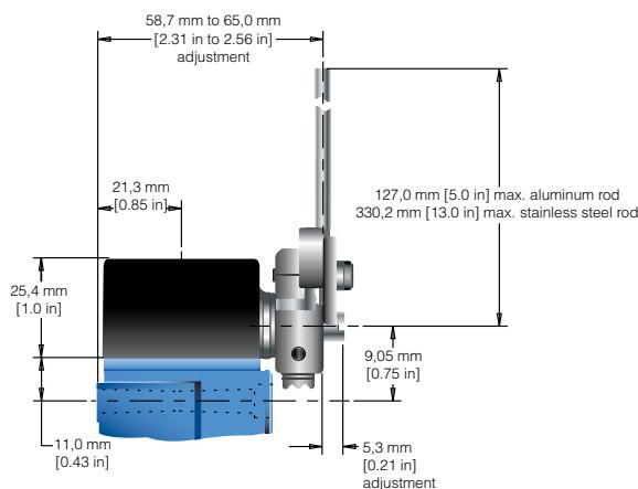
**Figure 9. LSZ55 type levers cam tracking**
