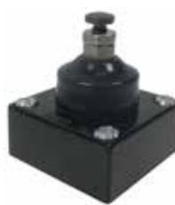
**LSV - Adjustable top pin plunger:** Provides easy application and saves on installation time. The operating points of the switch can be adjusted from 52,8 mm to 59,3 mm [2.085 in to 2.335 in]. Seals are the same as the pin plunger. Momentary action.
