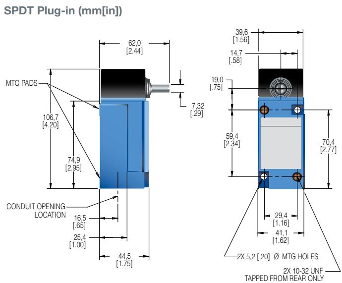
**Figure 3. MICRO SWITCH™ HDLS side rotary (double pole) dimensions**
