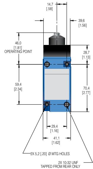
**Figure 11. MICRO SWITCH™ HDLS LSC Series (double pole plunger dimensions**
