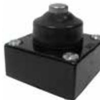
**LSC - Top pin plunger:** A corrosion-resistant steel plunger for in-line actuating motion. Oil-tight seals on plunger and between the operating head and housing keep out coolant, dust, and chips. Momentary action.
