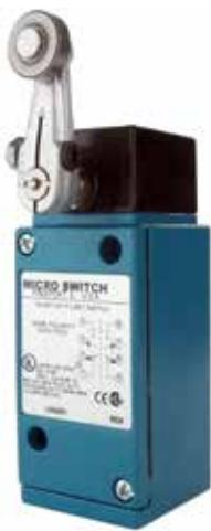
This series has a wide gap contact block that handles a higher make/break dc load. In addition, a special lever arm has a serrated shaft hole and a cap screw with locking nut for attaching the lever to the rotary shaft. This assures a firm grip on the operating shaft and positive retention of the lever adjustment.
