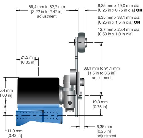
**Figure 8. LSZ54 type levers cam tracking**
