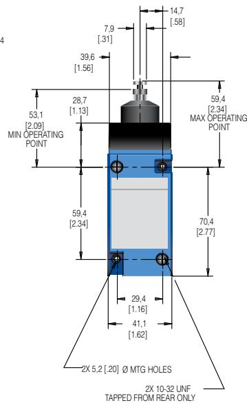
Figure 15. MICRO SWITCH™ HDLS LSV Series top adjustable plunger (double pole) dimensions
