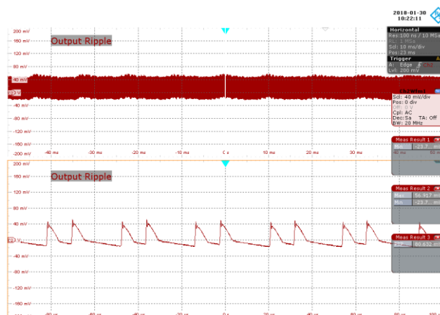
Figure 105 – 115 VAC 47 Hz, 75% Load. CH1: V_{OUT} , 40 mV / div., 10 ms / div. Zoom: 20 μs / div. Voltage Ripple ( V_{OUT(PK-PK)} ) = 80.6 mV).
