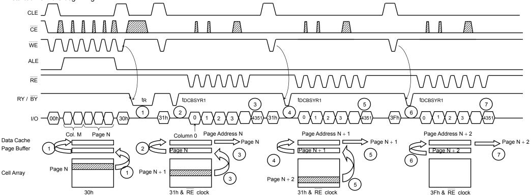
If the 31h command is issued to the device, the data content of the next page is transferred to the Page Buffer during serial data out from the Data Cache, reducing the t<sub>R</sub> (Data transfer from memory cell to data register).
