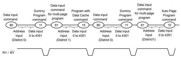
After either "15h" or "10h" Program command is input to the device, physical programing starts as follows. For details about Auto Page Program with Data Cache, refer to "Auto Page Program Operation with Data Cache".
