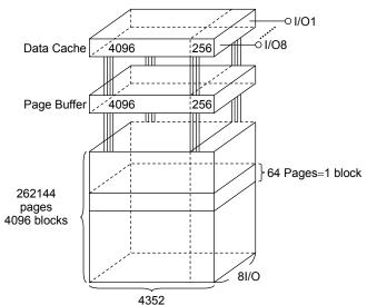
A page consists of 4352 bytes in which 4096 bytes are used for main memory storage and 256 bytes are for redundancy or for other uses.
