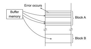
When an error happens in Block A, try to reprogram the data into another Block (Block B) by loading from an external buffer. Then, prevent further system accesses to Block A ( by creating a bad block table or by using another appropriate scheme).
