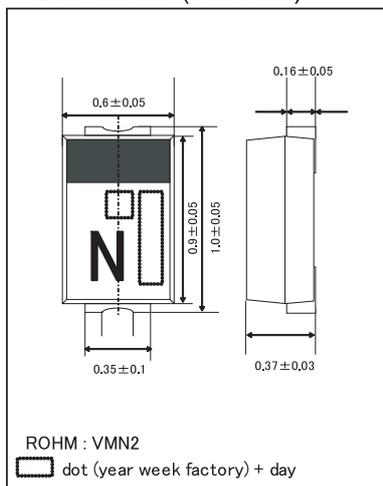
●Lead size figure (Unit : mm)
