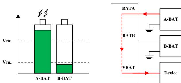
State 7: If  $V_{B-BAT} \leq V_{TH2}$ , A-BAT provides power all the time.
