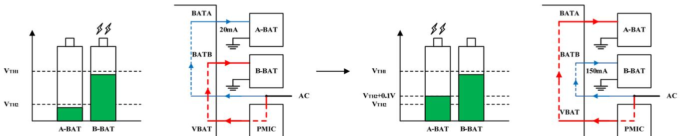
**State 3:** If  $V_{A-BAT} \leq V_{TH2}$  and  $V_{TH2} \leq V_{B-BAT} \leq V_{TH1}$ , B-BAT provides power. The PMIC charges up for B-BAT and IS31PW8200 provides small current (20mA) for A-BAT by internal charger at the same time. The battery source will not switch until  $V_{A-BAT}$  reaches  $V_{TH2}+0.1V$ .
