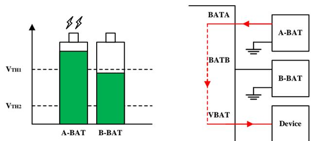
State 4: If  $V_{A-BAT} \geq V_{TH1}$  and  $V_{TH2} \leq V_{B-BAT} \leq V_{TH1}$ , A-BAT provides power.
