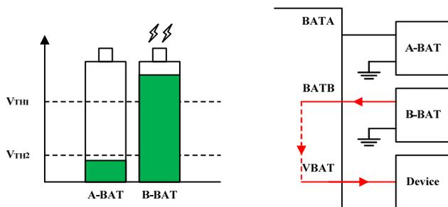
State 3: If  $V_{A-BAT} \leq V_{TH2}$  and  $V_{B-BAT} \geq V_{TH1}$ , switch to B-BAT providing power immediately.
