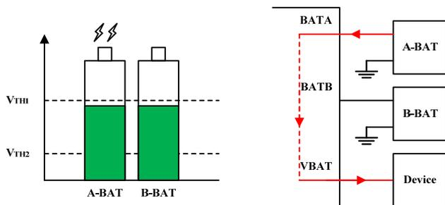
State 5: If  $V_{TH2} \leq V_{A-BAT} \leq V_{TH1}$  and  $V_{TH2} \leq V_{B-BAT} \leq V_{TH1}$ , A-BAT provides power.
