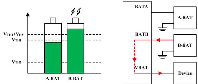
State 2: If  $V_{A-BAT} \leq V_{TH1}$  and lasts for  $t_D$  and  $V_{B-BAT} \geq V_{TH1} + V_{HY}$ , switch to B-BAT providing power.
