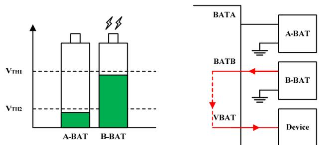
State 6: If  $V_{A-BAT} \leq V_{TH2}$  and  $V_{TH2} \leq V_{B-BAT} \leq V_{TH1}$ , switch to B-BAT providing power.
