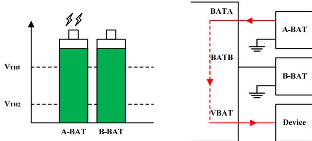
State 1: If  $V_{A-BAT} \geq V_{TH1}$  and  $V_{B-BAT} \geq V_{TH1}$ , A-BAT provides power.
