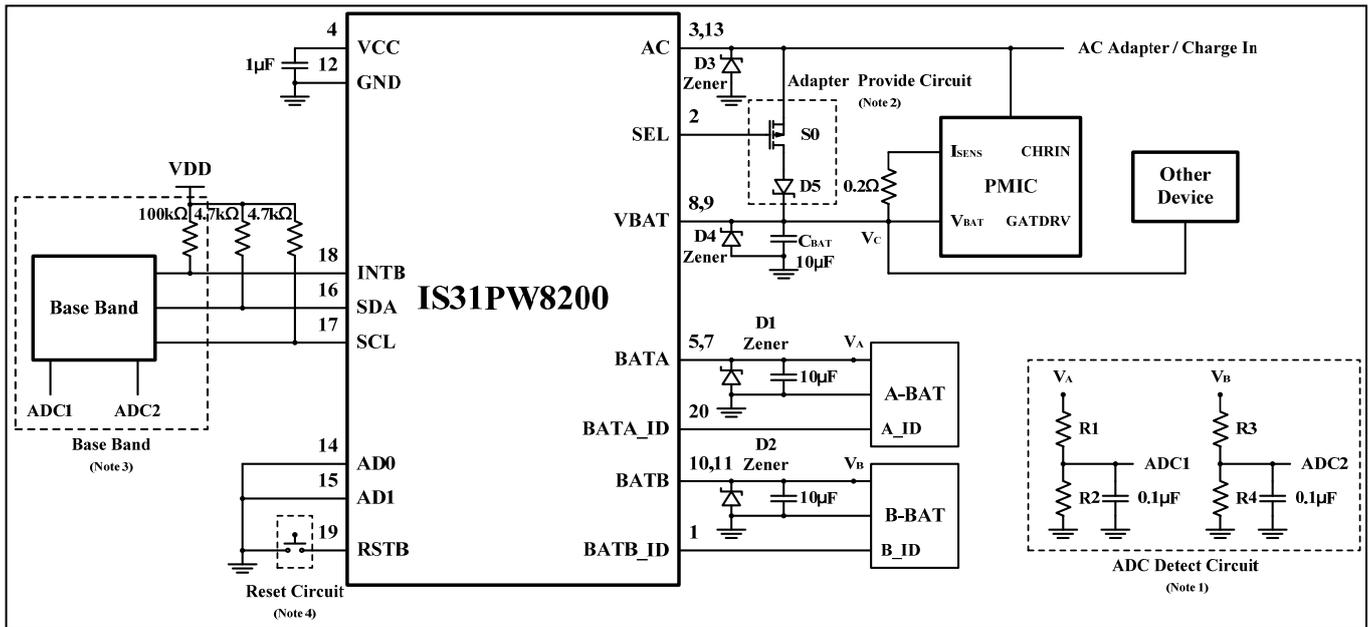
**Figure 2** Typical Application Circuit
