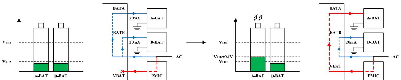
**State 5:** If  $V_{A-BAT} \leq V_{TH2}$  and  $V_{B-BAT} \leq V_{TH2}$ , dual batteries disconnect with VBAT. At this moment, the PMIC doesn't charge up any batteries and IS31PW8200 provides small current (20mA) for dual batteries by internal charger until one of batteries is charged up to  $V_{TH2}+0.1V$  and offer power by this battery.
