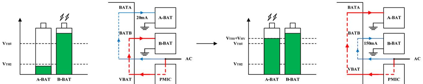
**State 1:** If  $V_{A-BAT} \leq V_{TH2}$  and  $V_{B-BAT} \geq V_{TH1}$ , B-BAT provides power. The PMIC charges up B-BAT and IS31PW8200 provides small current (20mA) for A-BAT by internal charger at the same time. The battery source will not switch until  $V_{A-BAT}$  reaches to  $V_{TH1}+V_{HY}$ .
