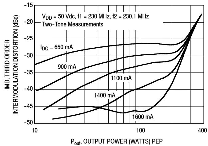
**Figure 13. Third Order Intermodulation Distortion versus Output Power**
