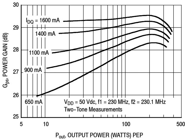
**Figure 12. Two-Tone Power Gain versus Output Power**
