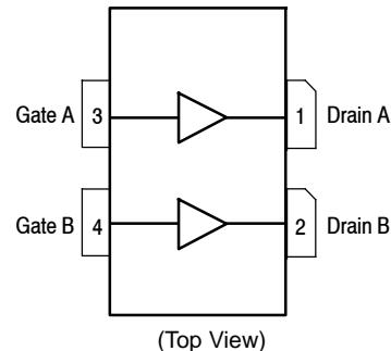
Note: The backside of the package is the source terminal for the transistors.
