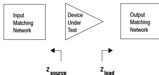
Figure 15. Series Equivalent Source and Load Impedance
