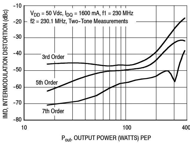
**Figure 10. Intermodulation Distortion Products versus Output Power**
