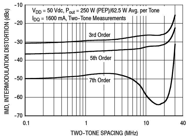
**Figure 11. Intermodulation Distortion Products versus Two-Tone Spacing**
