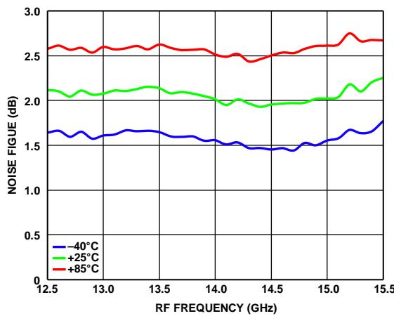
Figure 20. Noise Figure vs. RF Frequency at Various Temperatures
