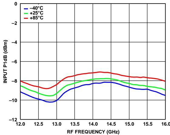
Figure 19. Input P1dB vs. RF Frequency at Various Temperatures
