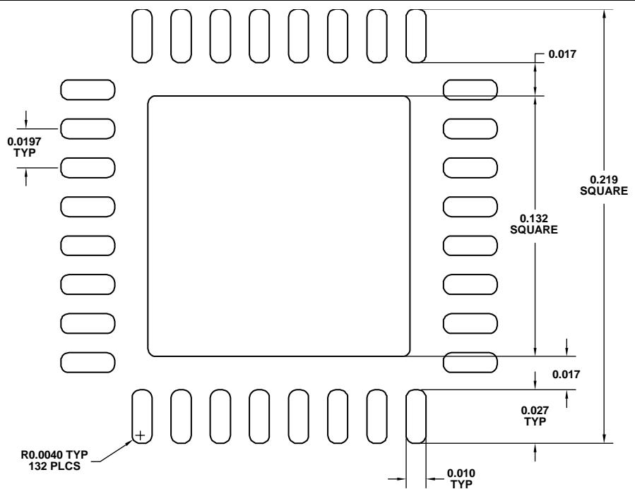
Figure 49. Solder Paste Stencil of the ADMV1010-EVALZ
