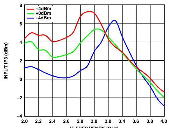
Figure 36. Input IP3 vs. IF Frequency at Various LO Powers
