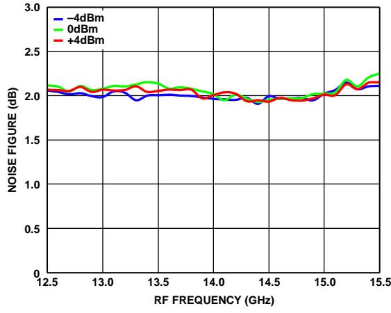
Figure 22. Noise Figure vs. RF Frequency at Various LO Powers
