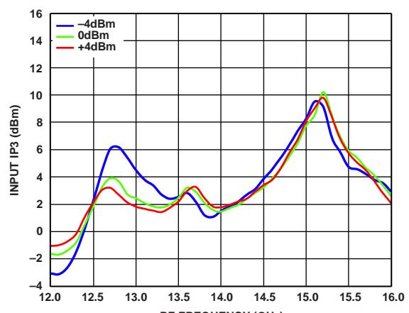
Figure 28. Input IP3 vs. RF Frequency at Various LO Powers
